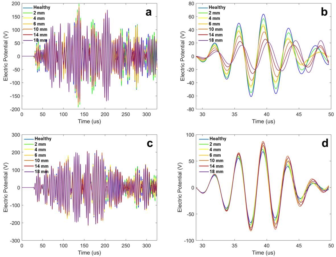
Figure 2. Indicative signals for the notched Al plate. (a) Full signal received at sensor 6 when sensor 2 is actuated, and (b) its first-arrival wave packet. (c) Full signal received at sensor 5 when sensor 1 is actuated, and (d) its first-arrival wave packet.
