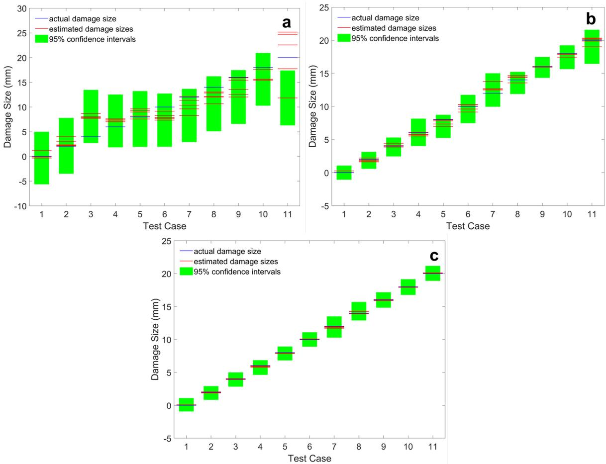
Figure 6. Indicative damage size estimation boxplots based on multivariate GPRMs: (a and b) 5 DIs used for two sets of three randomly selected paths; (c) 5 DIs used from three paths indicated by the non-parametric model.
