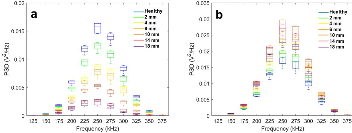
Figure 4. Indicative results of applying the non-parametric model onto actuator-sensor paths. Short Time Fourier Transform (STFT) plots for the signals of (a) damage-intersecting path 2-6 and (b) damage-non-intersecting path 1-5.
