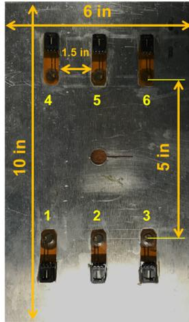
Figure 1. The notched Al plate experimental coupon used in this study.
