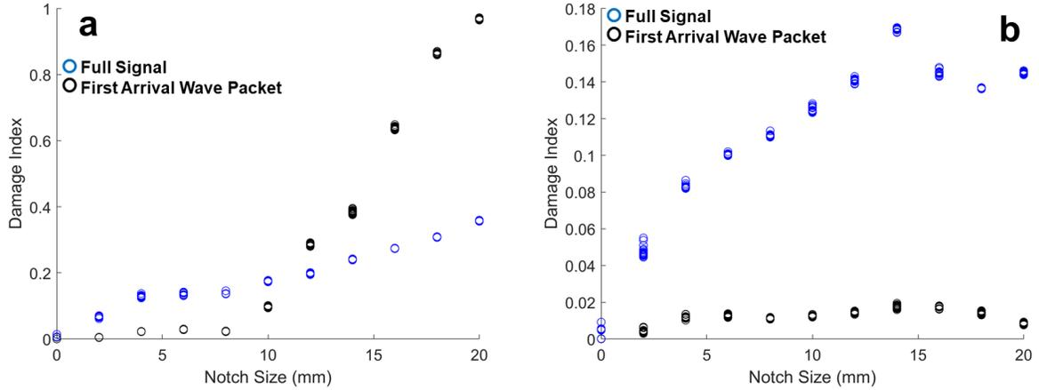
Figure 3. The evolution of the damage index [1] as applied to indicative actuator-sensor paths: (a) damage-intersecting path 2-6 and (b) damage-non-intersecting path 1-5.
