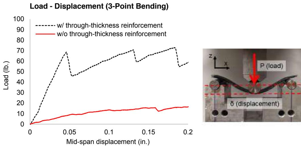
Figure 5. Load-displacement curve for the 3-point bending test comparing (dotted black line) samples with through-thickness reinforcements and (solid red line) samples without through-thickness reinforcements
