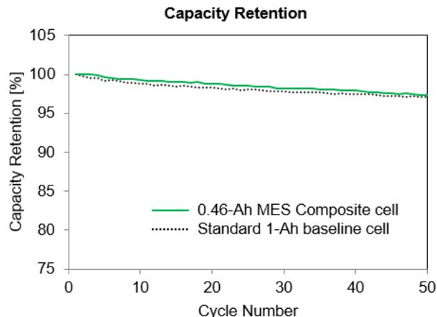
Figure 4. Capacity retention (retained capacity –vs- number of cycles) of the 0.46-Ah MES Composite single cell, in comparison with a 1-Ah standard baseline cell
