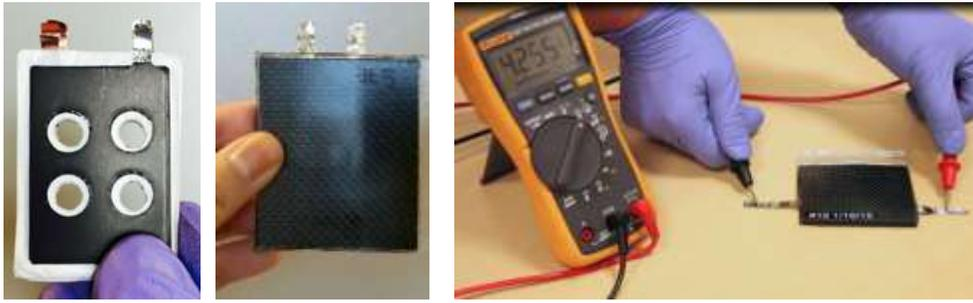
Figure 2. (left) Li-ion battery electrode stack with perforations for placement of through-thickness reinforcements; (center) finished MES Composite single cell; (right) 0.46-Ah MES Composite single cell showing 4.25V.
