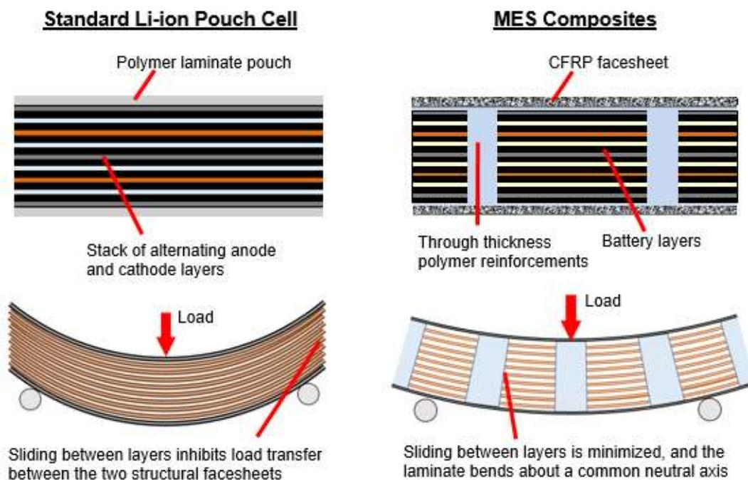
Figure 1. Comparison between standard Li-ion pouch cells (left) and MES Composites (right) – MES Composites employ through-thickness reinforcements which transfer mechanical loads between two structural facesheets and improve shear resistance of the battery core
