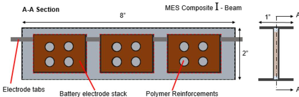
Figure 3. Configuration of the 3S MES Composite I-Beam module
