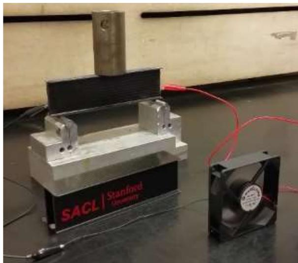
Figure 6. 3S MES Composite I-Beam module with nominal voltage of 11.1V, and 5.1Wh theoretical energy. The I-Beam can concurrently power a 12VDC fan while supporting a bending load.
