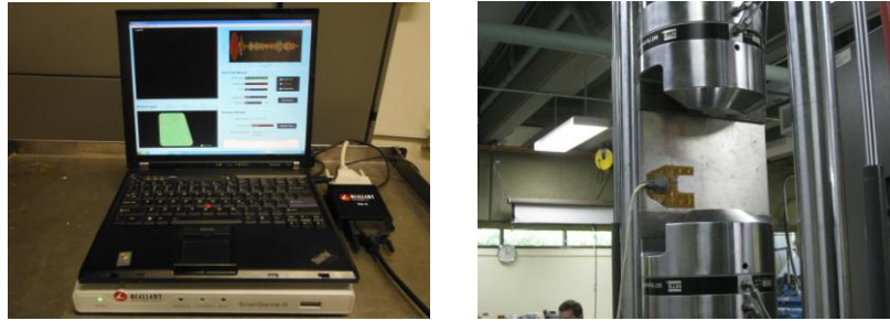
Figure 4: (a) Acellent’s ScanGenie data acquisition system with smartpatch software, and (b) MTS testing machine used for the fatigue and loads testing.
