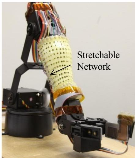
Figure 10 – Robotic arm with a stretchable network for state sensing
