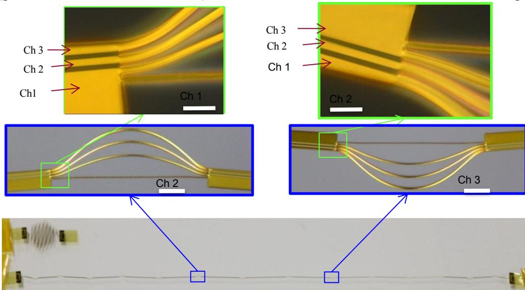
Figure 4 – Segmented interconnect section to reduce strain during expansion. 3 electrical channels are present for inter-nodal communication.
