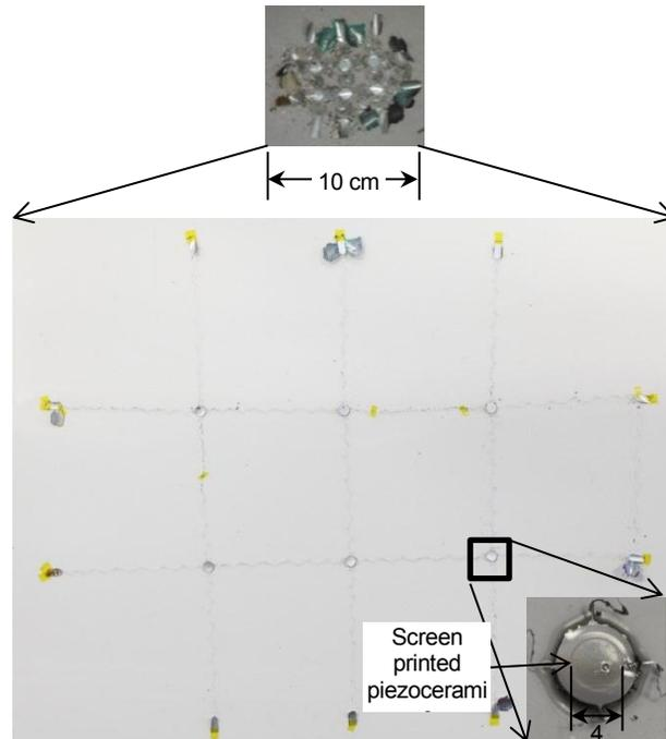
Figure 5 – Screen printed piezoceramics released onto polyimide and deployed on an expandable network. Before expansion (top) and after expansion (bottom). With a close up of a piezoceramic node (bottom right).
