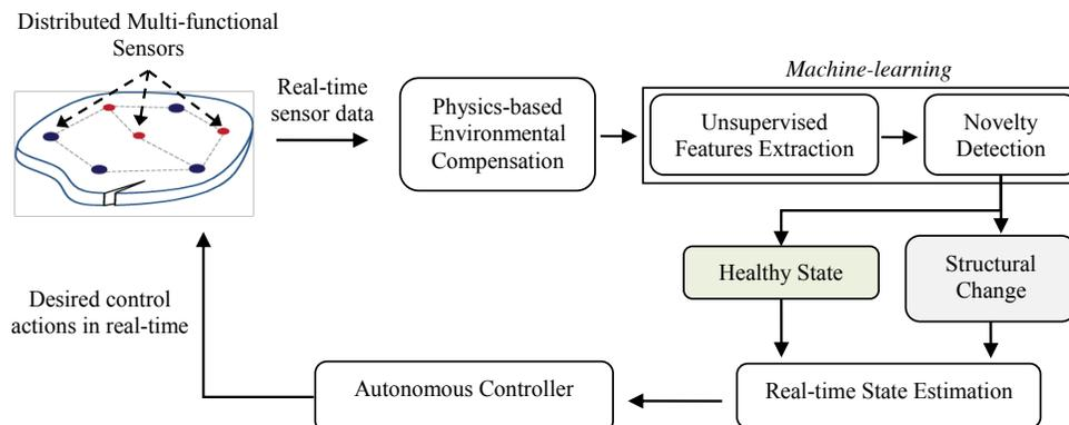
Figure 8 - Schematic for structural state identification and autonomous control actions in real-time using physics-based environmental compensation models and machine learning algorithms.
