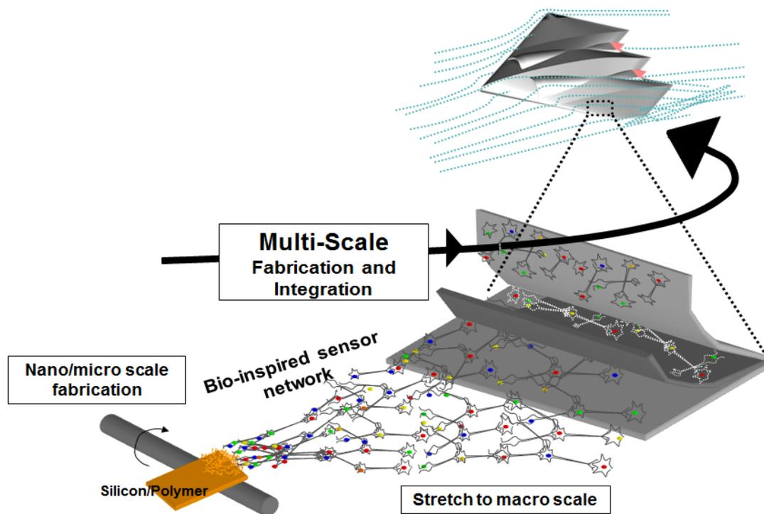
Figure 1 – Bio-inspired stretchable network concept for fabrication and deployment
