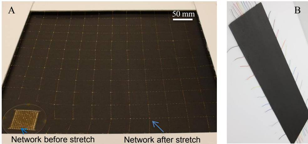
Figure 9 - A stretchable sensor network is embedded into carbon fiber composite materials.
