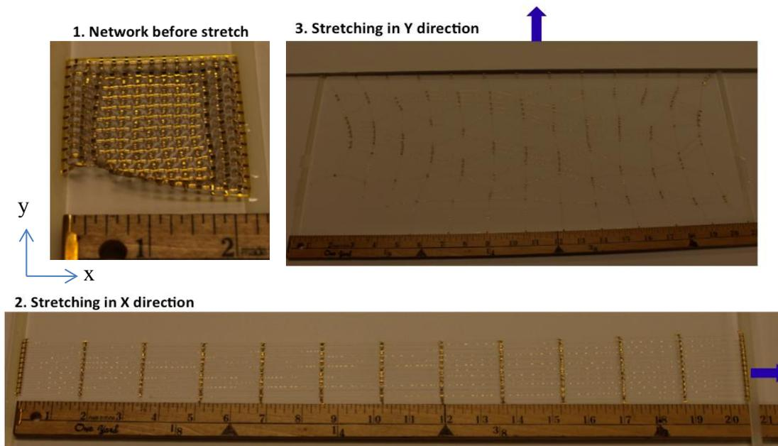
Figure 6 – Stretching of a 169 node sensor network
