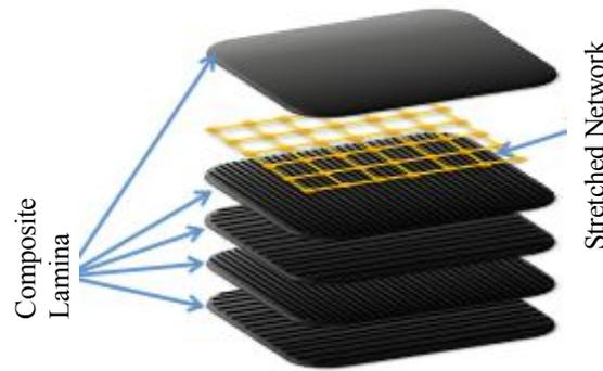
Figure 7 – Integration of a stretched sensor network into carbon fiber composite materials
