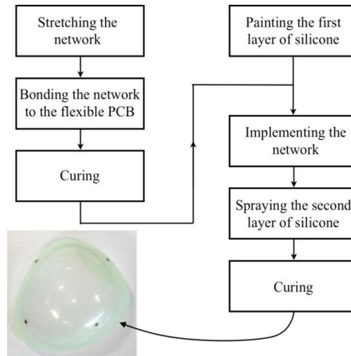
Figure 12 – Process for integrating stretchable networks into silicone membranes.
