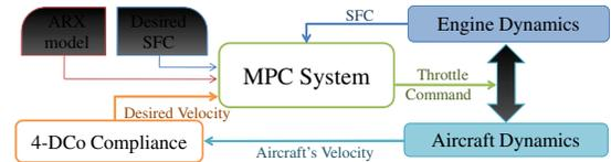
Fig. 4. The MPC based auto-throttle block diagram.
