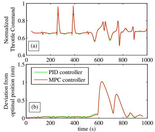
Fig. 7. Comparison of the proposed MPC and PID based controllers for an indicative turbulence-free cruise flight: (a) throttle command output and (b) 4DCo deviations (nautical miles, nm).
