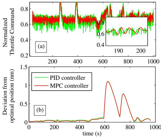
Fig. 8. Comparison of the MPC and PID based controllers for an indicative type A (low-level) turbulence cruise flight: (a) throttle command output and (b) 4DCo deviations (nautical miles, nm).
