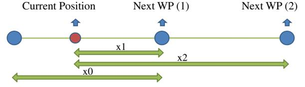
Fig. 1. The aircraft desired velocity at the current condition depends on WP(1) and WP(2). A component-velocity is calculated for each of these two WPs, dividing its distance from the aircraft with the remaining time-to-arrival. The desired velocity is a linear combination of the two component velocities.
