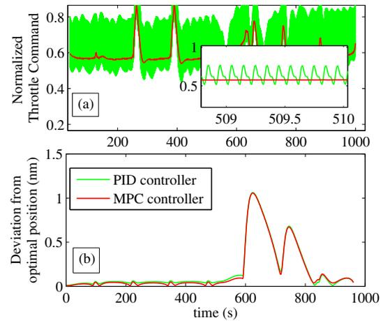
Fig. 9. Comparison of the MPC and PID based controllers for an indicative type B (high-level) turbulence cruise flight: (a) throttle command output and (b) 4DCo deviations (nautical miles, nm).
