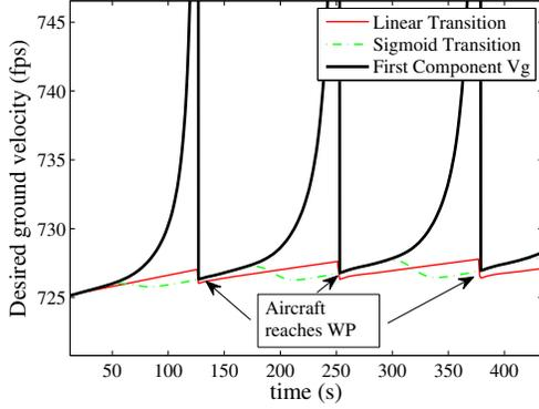
Fig. 2. Methods for defining the desired aircraft ground velocity.
