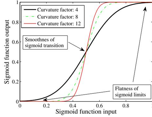
Fig. 3. The sigmoid function for various curvature factors.
