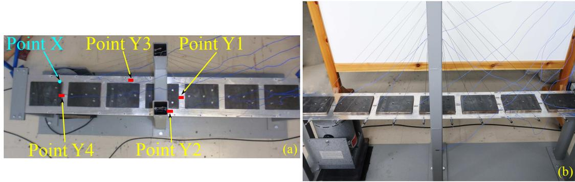
Figure 1: The scale cable-stayed bridge structure and the experimental set-up: (a) top-to-bottom view, and (b) general overview (force excitation at Point X and vibration measurement at Points Y1–Y4).
