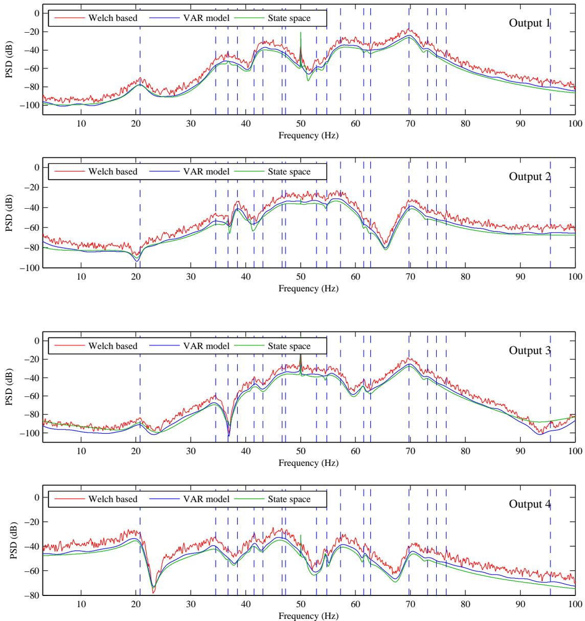
Figure 2: Non-parametric (Welch-based) and parametric (VAR(49) and SS(55) based) spectral estimates. The dashed vertical lines indicate actual structural modes.
