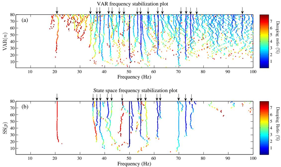
Figure 4: Frequency stabilization diagrams for  $\text{VAR}(n)$  and  $\text{SS}(p)$  type models.
