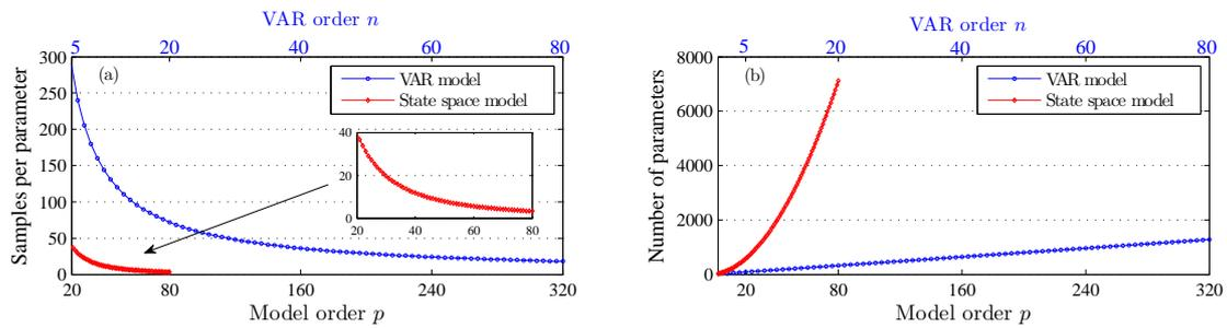
Figure 6: Model parsimony for VAR( $n$ ) and SS( $p$ ) type parametric models: (a) samples per parameter (SPP) and (b) number of parameters for increasing model order.
